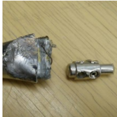
EOD Charge SSD, 20g Semtex10, 14 cm stand-off, mechanical fuze of mortar grenade, breaking
