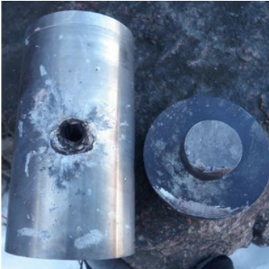
EOD Charge Cu, 50 g Semtex10, 14 cm stand-off, TNT-filled pipe IED, deflagration
