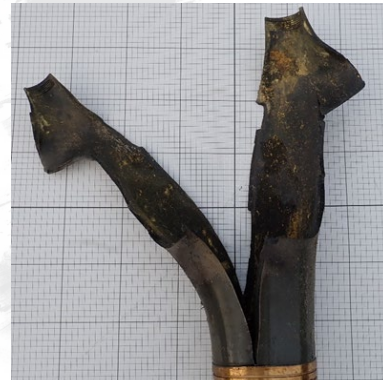
EOD Charge Cu, 60g PENO, 14cm stand-off, 155mm artillery grenade, deflagration
