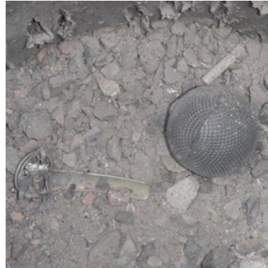
EOD Charge SSD, 20 g PENO, 14 cm stand-off, hand grenade, breaking
