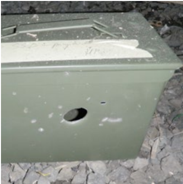
EOD Charge SSD, 40 g Semtex10, 100 cm stand-off, metal case, penetration
